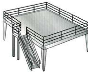
**Freestanding Mezzanines** are supported by framing members connected to the primary floor by columns alone, creating optimum usable space above *and* below.
